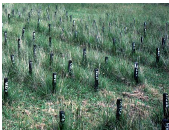
A long-term field test of treated stakes
