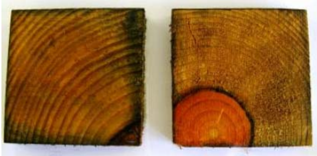
Test showing heartwood (red) and copper penetration (blue) in two pine posts (left: freshly treated, sapwood 120% moisture content, right: above ground section of failed post)
