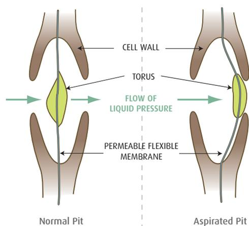
Pit aspiration with spruce generally increases during forced drying conditions such as kiln drying as opposed to air-drying. High temperature kiln drying to low moisture contents will dry the timber to what may appear to be an ideal moisture content for preservation but in terms of preservative penetration, this can be off-set due to an increased level of pit aspiration.
