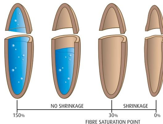
It is important to understand that timber moisture content relates to the dry weight of timber and freshly felled timber can have moisture contents as high as 150%. To dry spruce from 150% mc to 28% mc requires the removal of over 500 litres of water per cubic metre of timber. However, as detailed in section 6, the spruces may be more receptive to treatment at a moisture content above 28%.
