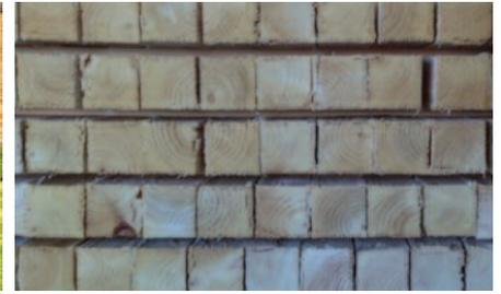
Sawn and incised 75mm x 75mm posts awaiting commercial impregnation for ground contact use class 4
