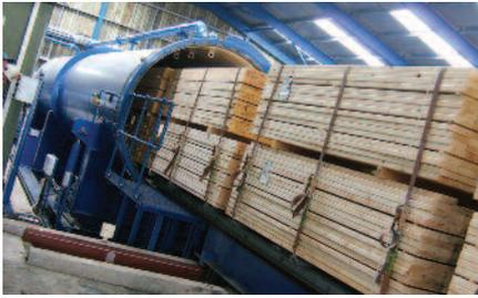
Treatment of posts will be to recommended retentions to achieve BS8417 UC4 15 years specification. Some batches will be treated at higher retentions to provide comparative data.
